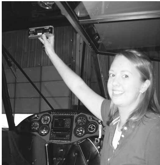
Figure 6-2 - Leveling the Aircraft
